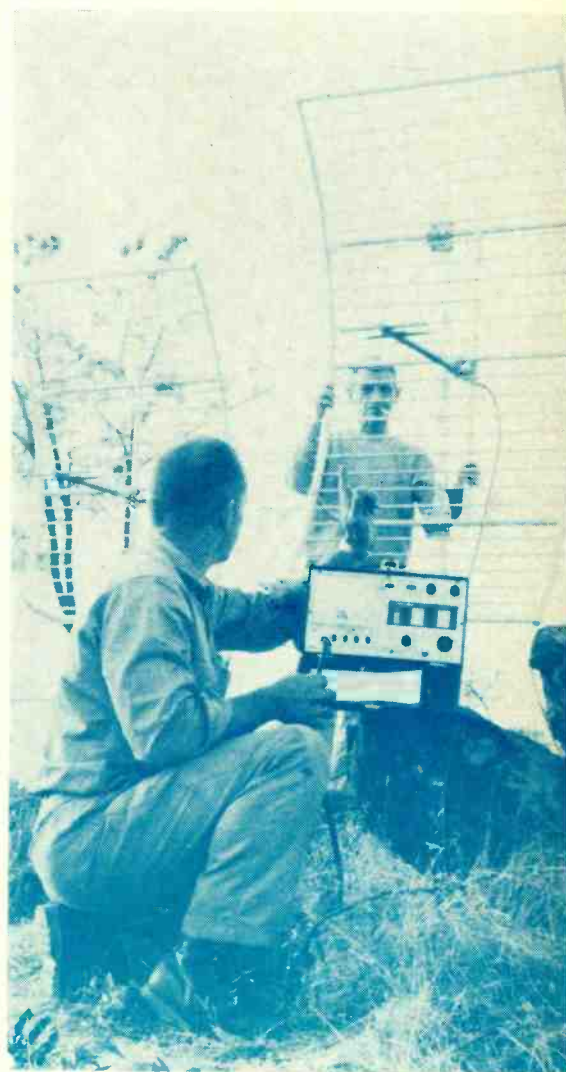
Field strength meter puts the finger on critical antenna location for Channel 30 Fresno.
